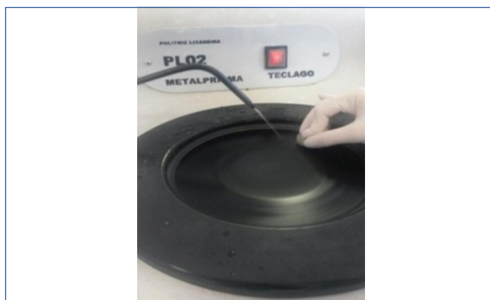
[Table/Fig-2]: The buccal surfaces were sanded under digital pressure.
